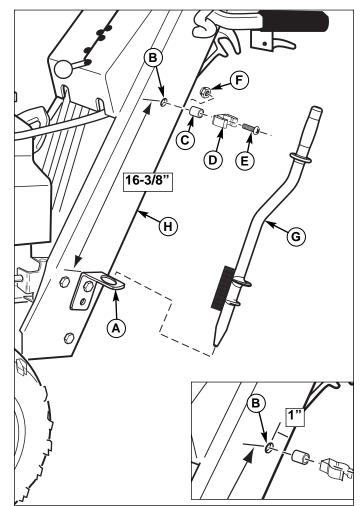
Figure 4. Mounting Clean-Out Tool (Channel Handle) F. Locknut, #10-24
